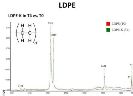
Figure 5. Spectral profile of LDPE, as determined by ATR-FTIR. The plot shows the results of the spectra spectrum of the control (LDPE-K, on the top) and the sample with the bacterial inoculate (LDPE-I18, on the bottom) at T4, superimposed to the spectrum of LDPE microplastics at the beginning of the experiment (T0).
