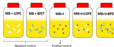
Figure 2. Scheme of the experimental conditions of the biodegradation experiment, in which 10 particles of each polymer (LDPE or BPET), were inoculated (10%) with different marine bacterial consortiums. A negative and positive control were used, where either no inoculum, or no MPs were added, respectively. I stands for inoculum; MB for marine broth; LDPE for low-density polyethylene; and BPET for biodegradable polyethylene terephthalate.
