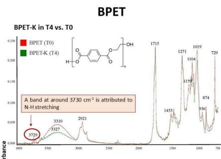
Figure 6. Spectral profile of BPET, as determined by ATR-FTIR. The plot shows the results of the spectra of the control (BPET-K, on the top) and the sample with the bacterial inoculate (BPET-I18, on the bottom) at T4, superimposed to the spectrum of BPET microplastics at the beginning of the experiment (T0).
