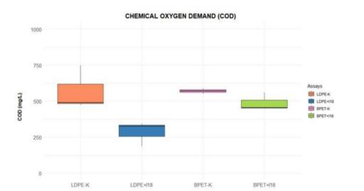
Figure 7. Representation of COD measured at the end of the experiment (after 45 days of incubation) for 5 LDPE and BPET particles. K stands for the controls and I18 for the samples inoculated with marine bacteria (inoculum 18).
